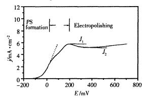
Fig 3 Current-potential curve of the p<sup>+</sup> silicon sample in 1% HF solution with potential sweep rate of 2 mV/s
