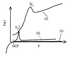
YFig 2 The typical i~V cures for silicon dissolved in HF(3), alkaline (2) and non-fluoride, non-alkaline solutions (1)
