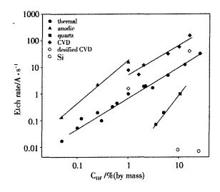
Fig 5 Etch rate of different silicon oxides as a function of HF concentration
