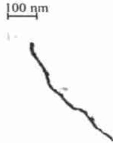
Fig. 2 TEM image of the single Au nanowire after completely removing of the AAO template
