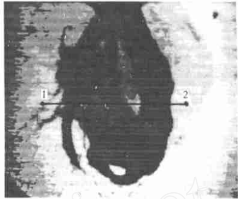
Fig. 6 CCD image of pitting corrosion of passive film on Rebar electrode in simulated cement pore solution ( \text{pH} = 12.5 ) containing 10% NaCl. The black region represents corrosive pit.
