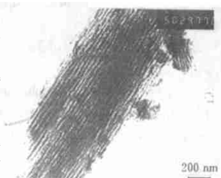
Fig. 1 The cross section of \text{Cd}_{0.67}\text{Zn}_{0.33}\text{S} nanowire arrays deposited in the matrix of anodic aluminum oxide (AAO)
