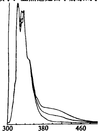
Fig. 5 Fluorescence spectra of naphthalene in the presence of \beta -Cyclodextrin and urea [naphthalene] = 1.6 \times 10^{-4} mol / l; [ \beta -CD] = 5 \times 10^{-3} mol / l; [urea] = 2.0 mol / l. Excitation wavelength: 280nm. Spectra normalized at 337nm. 1. Naphthalene; 2. Naphthalene / \beta -CD / urea; 3. Naphthalene / \beta -CD.
