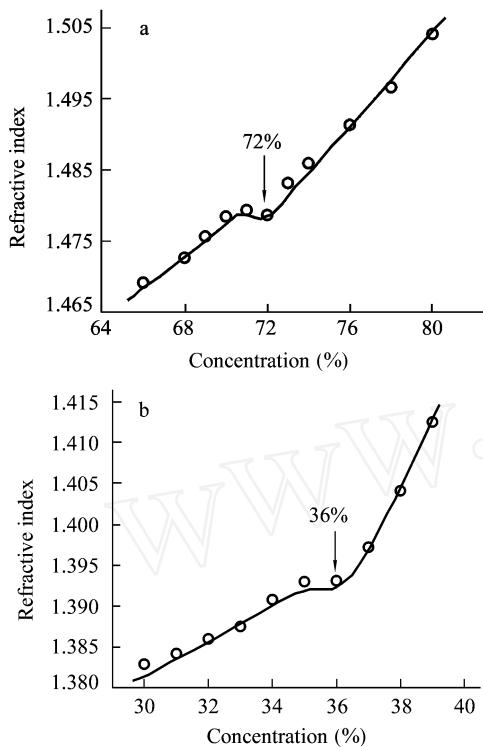
Fig. 6 Measurements of  $c^*$  by refractometry for a CS1/water solution (a) and a CS2/water solution (b)
