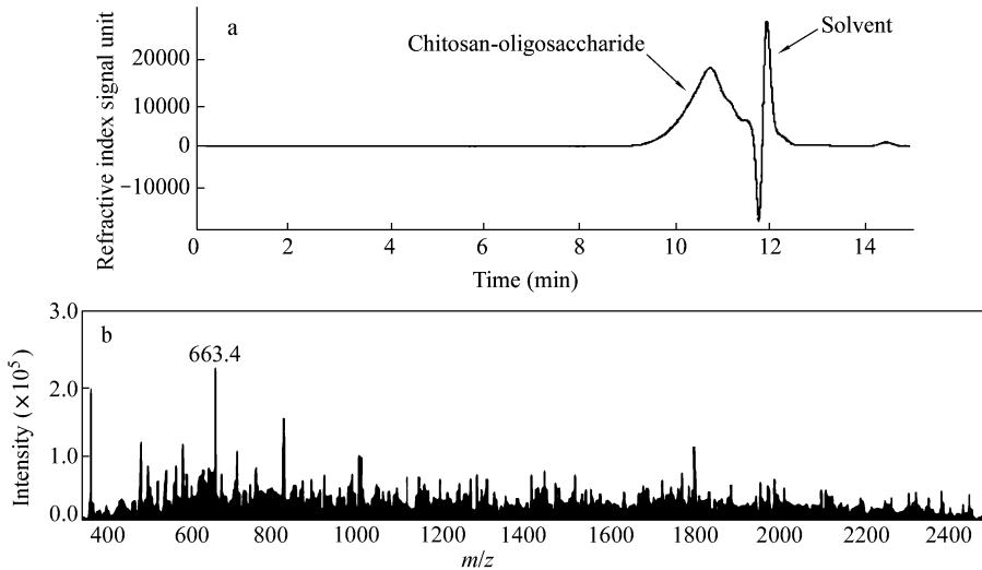
Fig. 2 GPC trace (a) and mass spectra (b) of CS1
