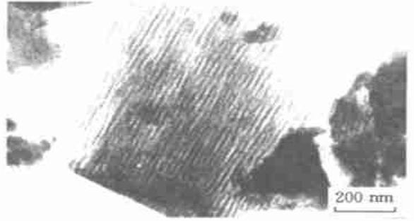
Fig 1 A TEM image of cross section of Ni nanowires array in porous alumina
