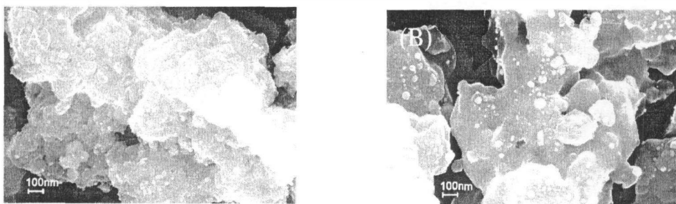
图4 不同温度下焙烧的 \text{Ag}/\text{TiO}_2 催化剂的SEM结果 Fig.4 SEM images of \text{Ag}/\text{TiO}_2 calcined at different temperature A-400 °C; B-500 °C
