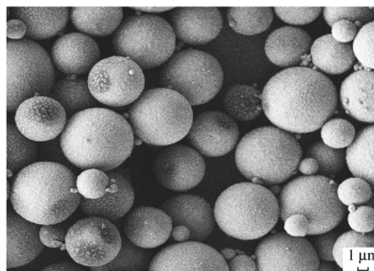
图 3 改良悬浮聚合法制备的磁性 PVAc 微球的 SEM 照片 Fig.3 SEM photograph of magnetic polyvinyl acetate (PVAc) microspheres prepared by the modification suspension polymerization
