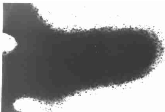
Fig. 1 Transmission electron micrograph ( \times 20\,000 ) of D01 biomass contacted with \text{Pt}^{4+} for 24 h.
