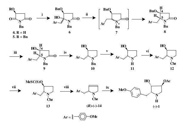
**Scheme 1.** Reagents and conditions: i) p-MeOC6H4CH2MgCl, THF, -15 °C ~ -10 °C, 94.5 %; ii) BF3 •OEt2, Et3SiH, -78 °C, 94.8 %; iii) H2, 1 atm, 10 % Pd/C, EtOH, 100 %; iv) LiAlH4, THF, reflux, 90 %; v) H2, 1atm, 20 % Pd(OH)2/C, EtOH, r.t.; vi) CbzCl, Et3N, CH2Cl2, r.t., 77 % over two steps; vii) NaH, THF, imidazole, 65 °C; CS2, 60 °C; MeI, 60 °C, 72 %; viii) neat, 190 °C, < 10 mmHg, 87.3 %; ix) ref. 8h.
