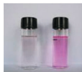
Fig. 1 Comparison of dRB-AE solution ( 1 \text{ mg ml}^{-1} ) in DMF containing triethylamine (TEA) (3%, v/v) before (left) and after (right) addition of diethyl chlorophosphate (100 ppm).
