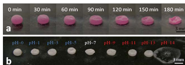
Fig. 7 (a) Digital photographs illustrating the effect of water evaporation on the shape of a liquid marble colored with Rhodamine B (20 ppm) after being placed on Petri dish at ambient temperature and 50% relative humidity and (b) effect of varying the solution pH on the stability of liquid marbles placed on Petri dish for 120 min.
