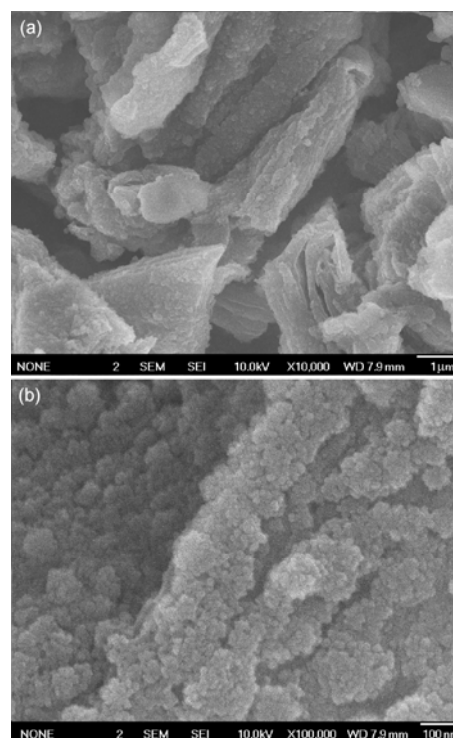
Figure 7 SEM images of the GNS electrode after 15 charge-discharge cycles.
