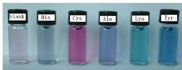
Fig. 1 Color changes of aqueous solutions of MOP (blank, 2.50 \times 10^{-5} M; buffered at pH 7.4 with 0.02 M phosphate buffer) with various L-amino acids ( 5.00 \times 10^{-4} M).
