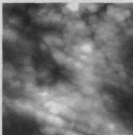
Figure 3 AFM image of a cross section of single bead nickel hydroxide (area 1\ \mu\text{m} \times 1\ \mu\text{m} )
