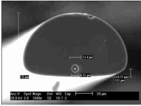
图 4 腐蚀 5 min 后的 D 形光纤截面扫描电镜照片 Fig. 4 Scanning electron microscope image of the D-shape fiber after etching of 5 minutes
