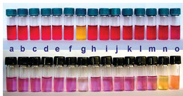
Fig. 2 Colour responses of (top) MoP and (bottom) AbP toward a variety of anions in aqueous solution at pH 7.4. [ CPAB ]: 1.0 \times 10^{-5} mol L ^{-1} ; anions ( 1.0 \times 10^{-4} mol L ^{-1} , from a to o): blank, F ^{-} , Cl ^{-} , Br ^{-} , I ^{-} , NO _3^{-} , SCN ^{-} , NO _2^{-} , SO _4^{2-} , HCO _3^{-} , PhCO _2^{-} , CH _3 CO _2^{-} , CN ^{-} , S ^{2-} and SO _3^{2-} ; pH buffer: 0.02 mol L ^{-1} phosphates.
