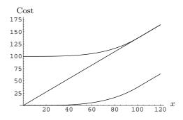
Notes. The bottom curve plots C(x, s), the present value of all future investment outlays incurred by the incumbent, when s = 100. The middle curve plots cx + C(x, x), the present value of all costs incurred by an entrant which replaces the network with one which is efficiently-configured. The top curve plots cs + C(x, s), the present value of all costs incurred by an entrant which replicates the network. In all cases, c = 1,  $\mu = 0$ ,  $\sigma = 0.1$ , r = 0.05 and  $\lambda = 0$ .
