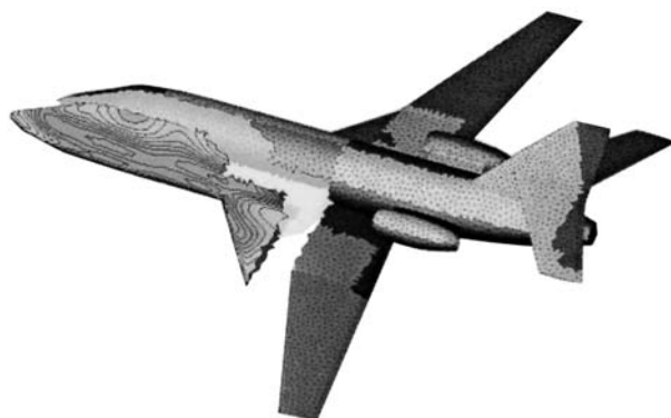
FIGURE 5. An extract of a solution of Maxwell equations on a perfectly conductive airplane \Gamma and the partitioning into 8 processes.
