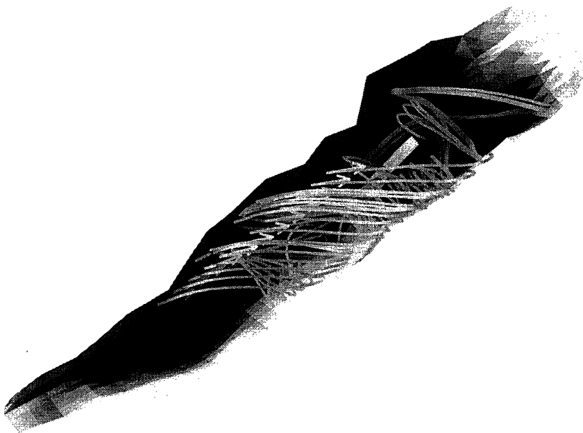
Figure 10: Streamlines in lake Neuchâtel, flow after 12h.
