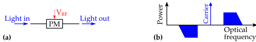
Fig. 1.11. (a) Structure of an phase modulator; PM: phase modulator. (b) Optical spectrum of a phase-modulated signal, comprising a carrier and two modulation sidebands in antiphase.
