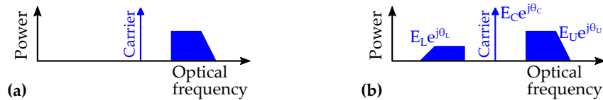
Fig. 1.12. Optical spectrum of (a) an SSB-modulated signal. (b) a signal modulated with a complex modulation type, where the amplitude and phases of the carrier and sidebands can be independently adjusted.
