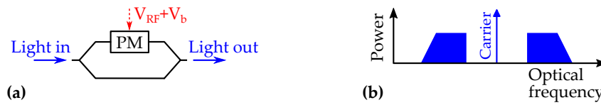
Fig. 1.10. (a) Structure of an intensity modulator; PM: phase modulator. (b) Optical spectrum of an intensity-modulated signal, comprising a carrier and two modulation sidebands in phase.
