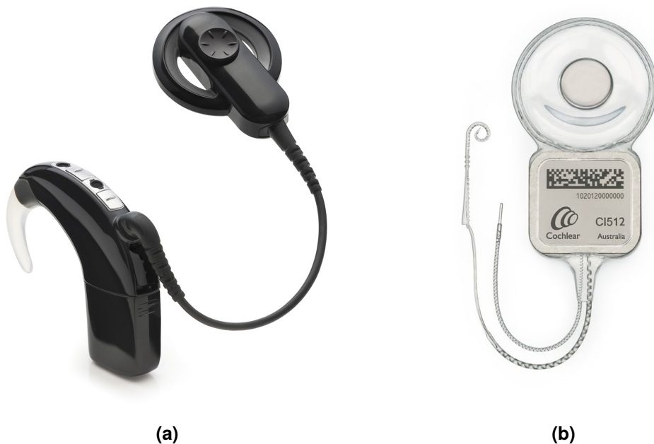
Figure 3.2: The Nucleus 6 cochlear implant system by Cochlear Limited. (a) The external behind-the-ear unit, housing the battery, microphone, speech processor, and stimulus controller tethered to the external coil. (b) The cochlear implant proper, consisting of the internal coil, stimulator circuitry, return electrodes, and intracochlear electrode array. The external and internal coils are aligned using magnets. (Source: Cochlear Limited.)
