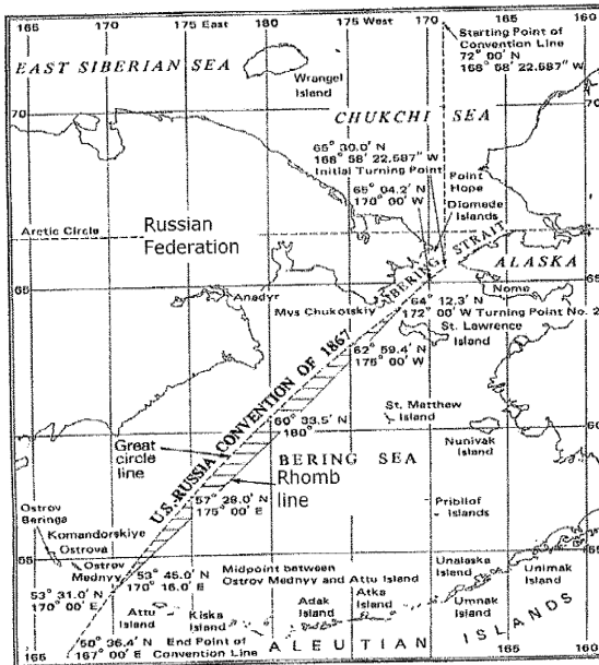
Figure 1 – Depiction of the Differences Between the Bering Sea Marine Boundary Using Rhomb and Geodetic Lines on a Mercator Projection
