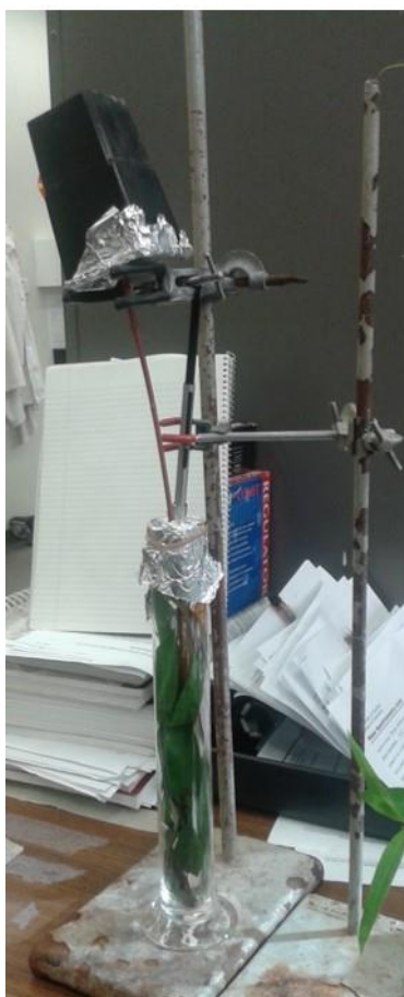
Figure S1. Experimental set-up used to extract headspace volatiles from Eucalyptus pilularis seedlings.
