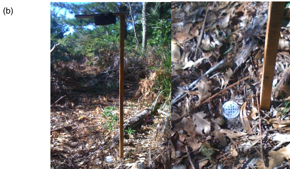
Figure S2. (a) Schematic of design for Experiment 2 and (b) photographs of camera and vial set-up.
