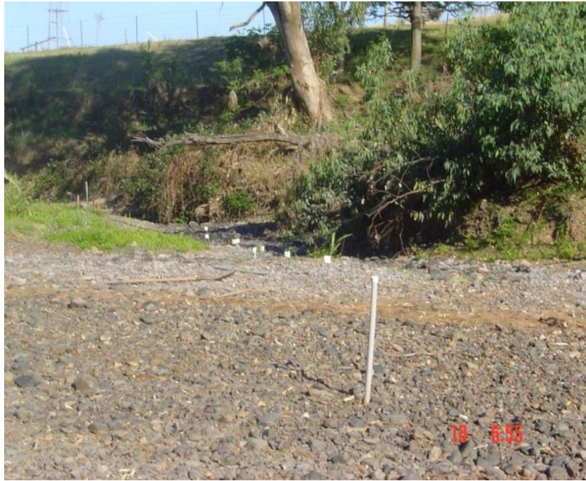
Figure 6-3. Location of in-stream piezometers used to delineate upwelling/downwelling process at the Ballantines transect (picture was taken during a dry spell of 2009).
