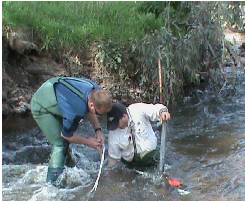
Figure 6-4. In the same locality as above, a T bar device was used to measure streambed temperatures at different depths. During flow events, it was not easy to find a plastic hose connected to the upper opening end of a buried piezometer pipe, which sticks out about 5 cm above the streambed
