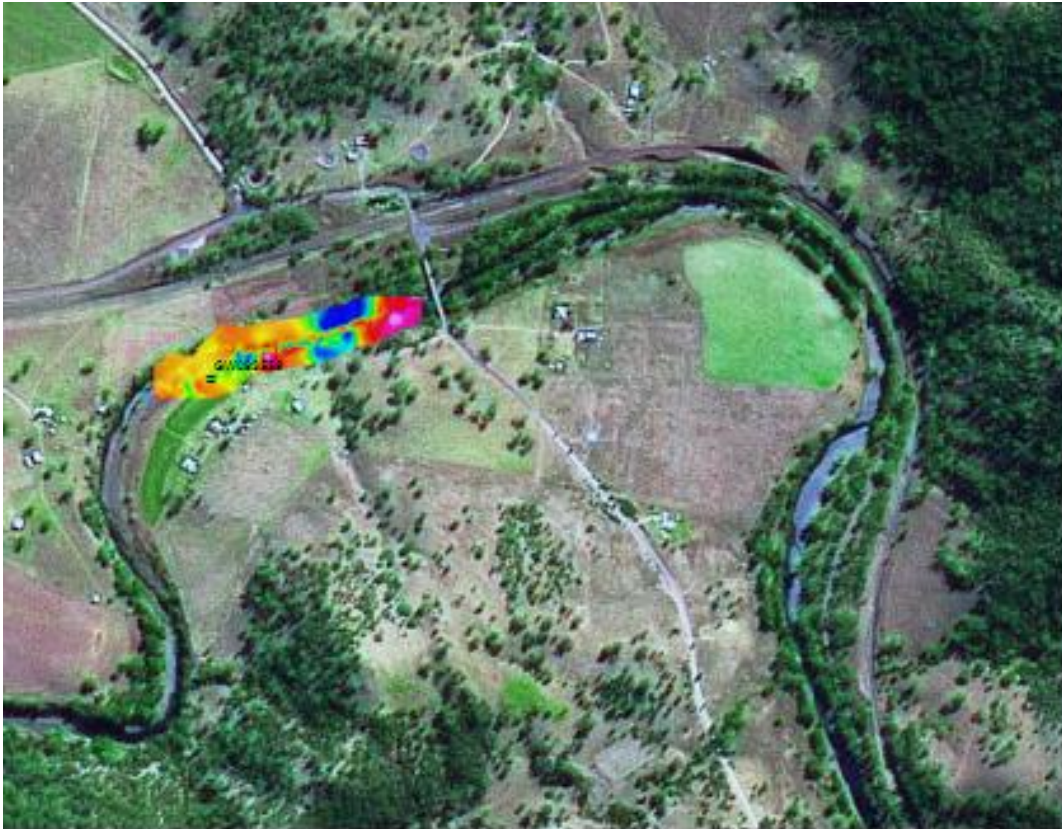
Figure 6-5. An EM-31 map for a dry spell period overlaid over a Spot 5 image for a riffle/pool system at the Ballantines transect.
