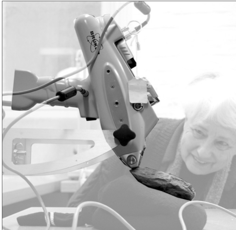
Figure 7.1: Non-destructive pXRF analysis of a ground edged hatchet – ensuring close and geometrically aligned contact between instrument and hatchet (Source: Grave et al 2012:1681)
