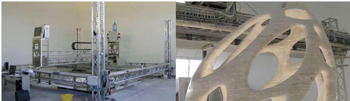
The d_shape printer (left) and pavilion printed with it (right) (Dini, 2010)
