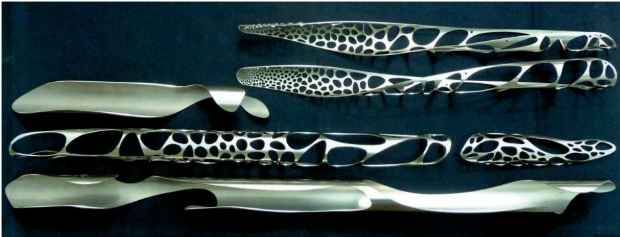
Steel tubes cut by Barkow Leibinger using a Trumpf laser-cutter (Barkow, 2010)
