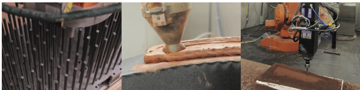
Robotically setting the pin mould (left), 3D printing ceramic slurry (centre) and robotically milling the surface (right) (Bechthold & Reinhart, 2011)
