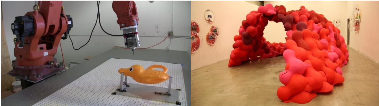
Robot arm used to cut pieces for Blobwall (left) 5 and the completed Blobwall (right) 6
