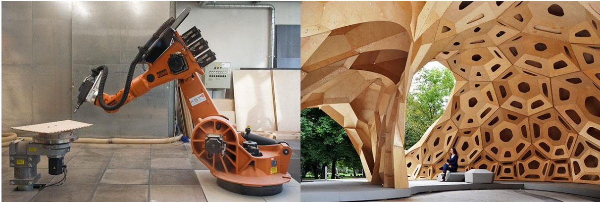
The industrial robot cutting complex finger joints (left) and the completed ICD|ITKE Pavilion (right) (Menges, 2011)
