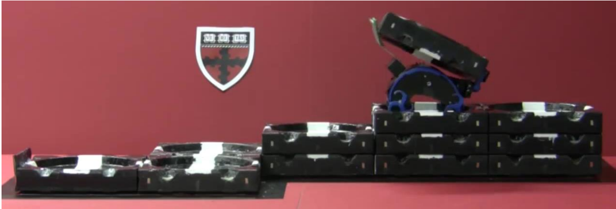
The autonomous robot used at Harvard University to constructs a staircase (Petersen, Nagpal & Werfel, 2011)
