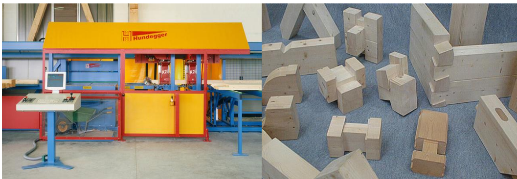
A Hundegger machine and some timber joinery produced by it (Hans Hundegger, 2010)
