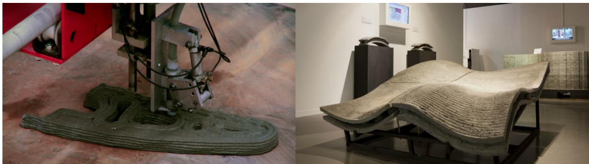
The 3D Concrete Printing Machine (left) and four panels fabricated with it (right) (Buswell, 2010)
