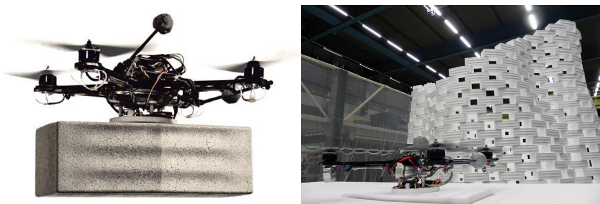
A quadrotor carrying a polystyrene module (left) 7 and a tower constructed from the modules (right) 8
