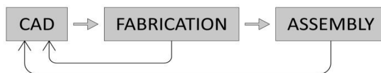
Figure 5.1 Separating the fabrication and assembly phases makes it difficult for students to respond to design issues that arise during the assembly phase.
