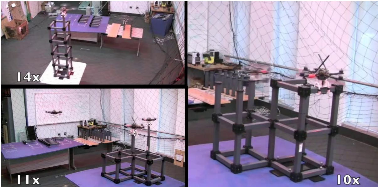
A team of three quadrotor robots used at Pennsylvania University to construct towers (Lindsey, Mellinger & Kumar, 2011)
