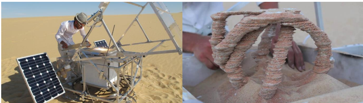
The Solar Sinter machine (left) and one of its creations (right) (Kayser, 2011)
