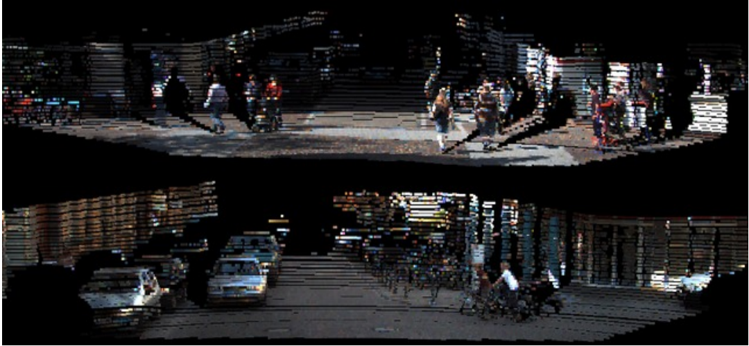
Figure 4.5: Visualisation of exemplary point clouds of the KITTI dataset coloured using information from the camera images.
