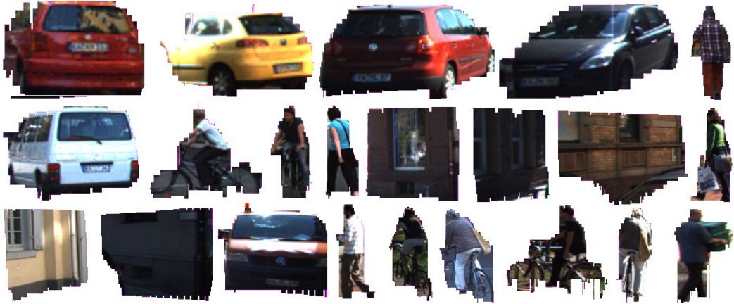
Figure 4.6: Exemplary image data corresponding to point cloud segments extracted from the raw Velodyne data. Shown are cars, pedestrians, cyclists and wall segments.
