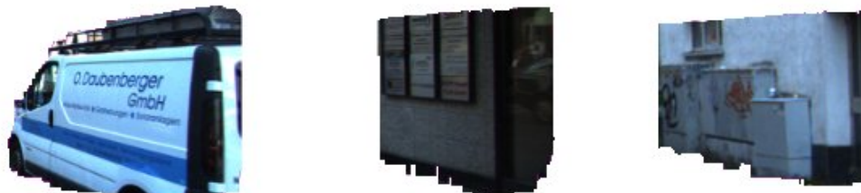
Figure 4.8: This shows one of the more common clustering mistakes, the side view of a car being clustered together with wall segments. Since only the planar side of the van is visible and both walls and van have rather uniform colour distributions this type of error is not surprising.
