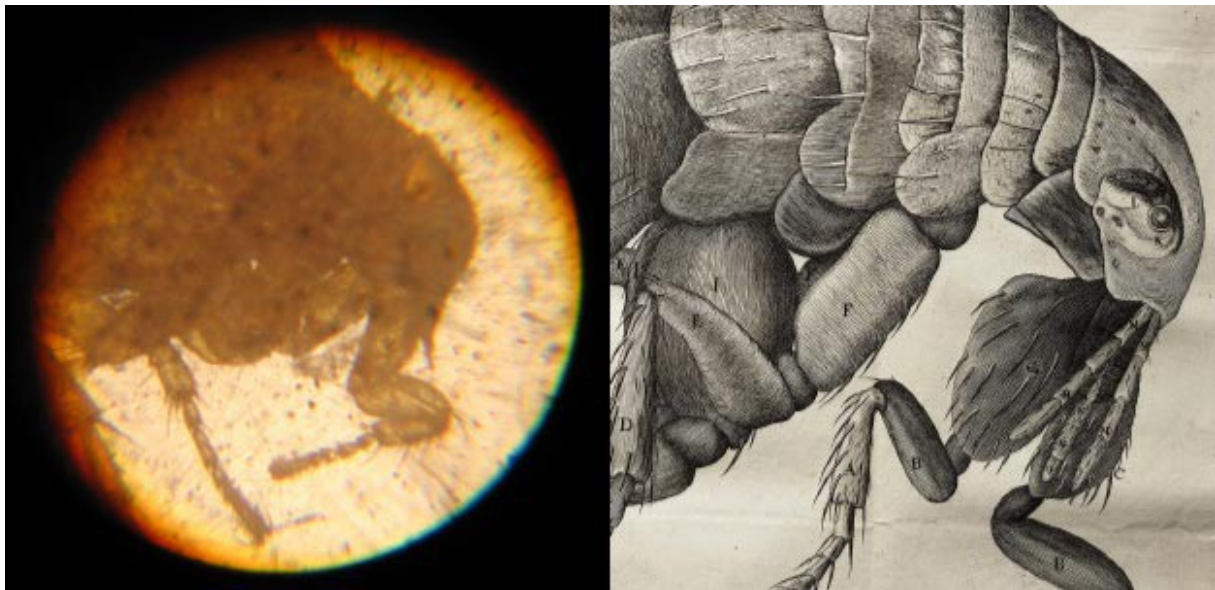
Figure 2.5: The slight chromatic aberration of a flea. The left image is a photo taken through an eighteenth century microscope, and shows a coloured halo, though not enough to completely obscure the image. (Image copyright The Whipple Museum of the History of Science, University of Cambridge [Wh.0080]). The right image, for comparison of the detail visible, is Hooke's flea from Micrographia , scheme 34 detail, opposite p. 210.
