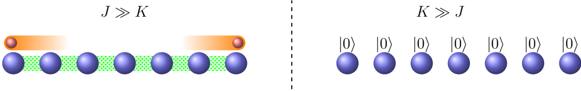
Figure 3.5: Ground states of two different phases of the Haldane chain, a nontrivial SP phase for J \gg K and a trivial phase for K \gg J .
