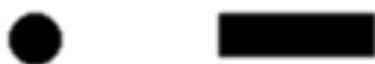
Figure 2: This is a ‘dit’ or ‘dot’ followed by a ‘dart’ or ‘dash’.
