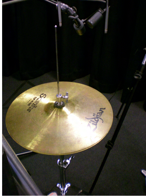
Figure 4.11: Microphone placement for the hi-hat. Note that the placement is slightly off-centre to avoid contact with the centre-rod.
