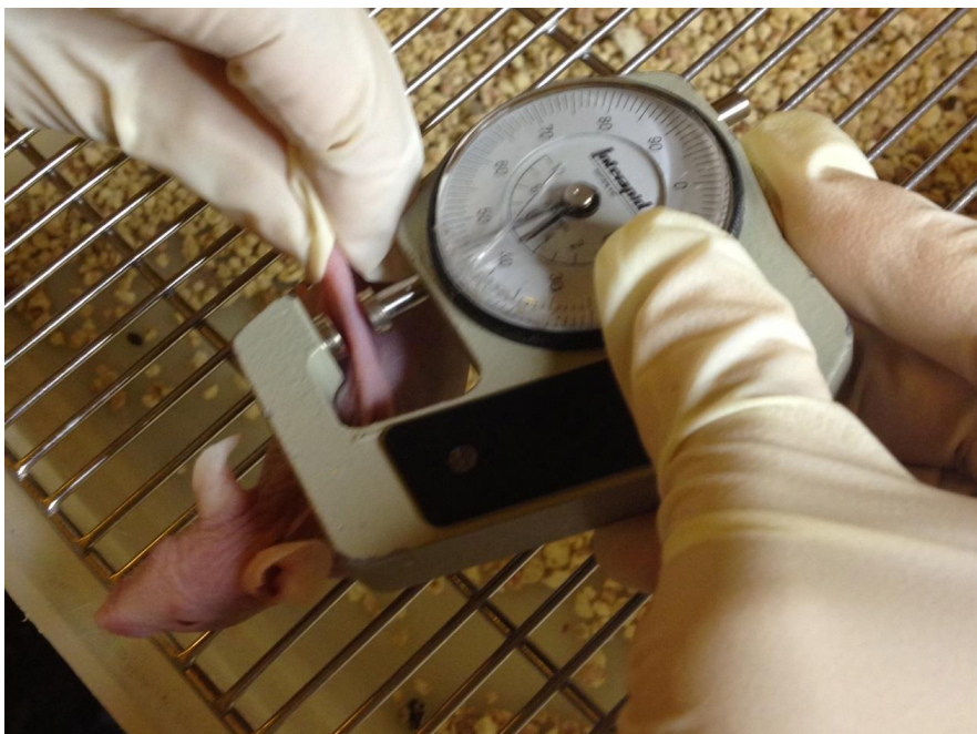
Figure 2.5 Measurement of dorsal skinfold thickness on a hairless Skh:Hr1 mouse using a spring micrometer
