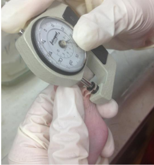
Figure 2.7 Measurement of ear swelling on a hairless Skh:Hr1 mouse using a spring micrometer
