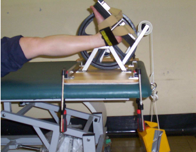
Figure 1. The device to measure passive ankle dorsiflexion.
