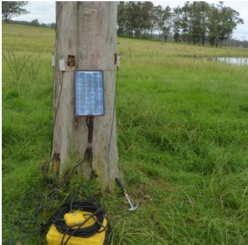
Figure 4.3: Sample tree, equipped with sap flow sensors, solar panel and logger/battery unit encased in a waterproof casing.
