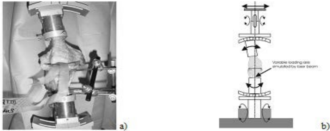
Figure 5. Mechanical testing for knee to simulate functional activities[12]
