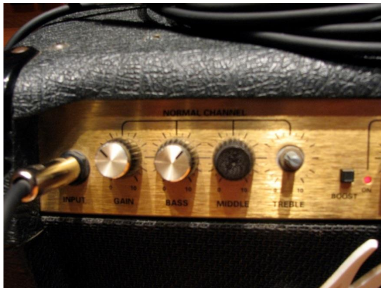
Figure 40: Clean channel of my 40 Watt 1995 Marshall 8040 Valvestate Amplifier. Note the missing treble knob and rubbed off marking on the middle tone knob. The gain channel was in a similar state of disrepair. 314
