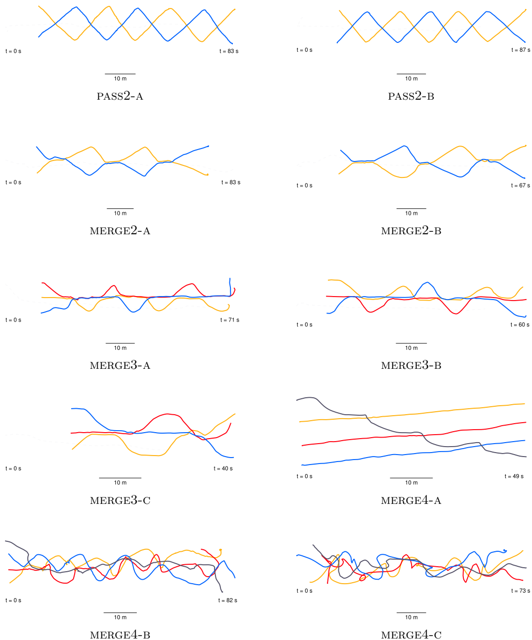
Figure 3.13 – Pedestrian interaction scenarios used to evaluate trackers. Each plot shows manually labelled object centroids, coloured per track, as seen from above. Targets move from left to right in the figures, and the start and end time is indicated. The sensor vehicle is manually driven approximately 10-15m behind the targets. In the 2 and 3 person interaction scenarios there is an extra track represented as a dashed grey line. This person is controlling the sensor vehicle and walks behind it, not interacting with the other people.
