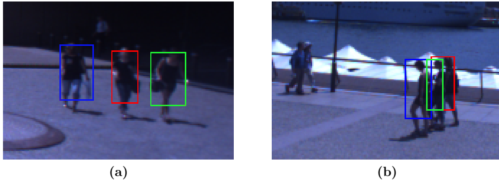
Figure 5.35 – Example of the changing target perspective during tracking. Early in the dataset, the targets are arranged parallel to the camera’s imaging plane, and so the appearance information from the three targets is well separated. Later during tracking, the targets are perpendicular to the image plane and the targets occlude each other.
