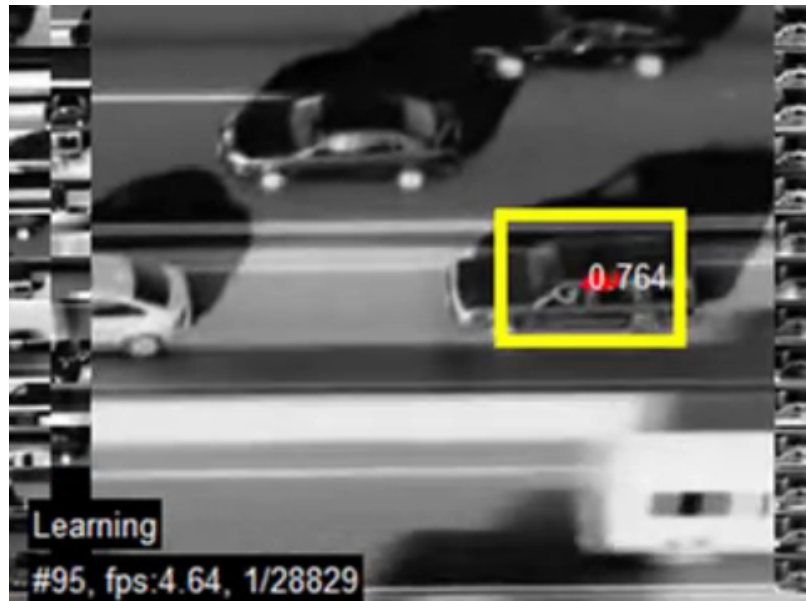
Figure 2.6 – Example of the TLD framework [49] being used to track a car from helicopter footage. Images on the right hand side of the frame are positive samples used to train the detector, whilst on the left hand side are the negative training examples. Image is from http://www.youtube.com/watch?v=Smh-HwtDHI8 .
