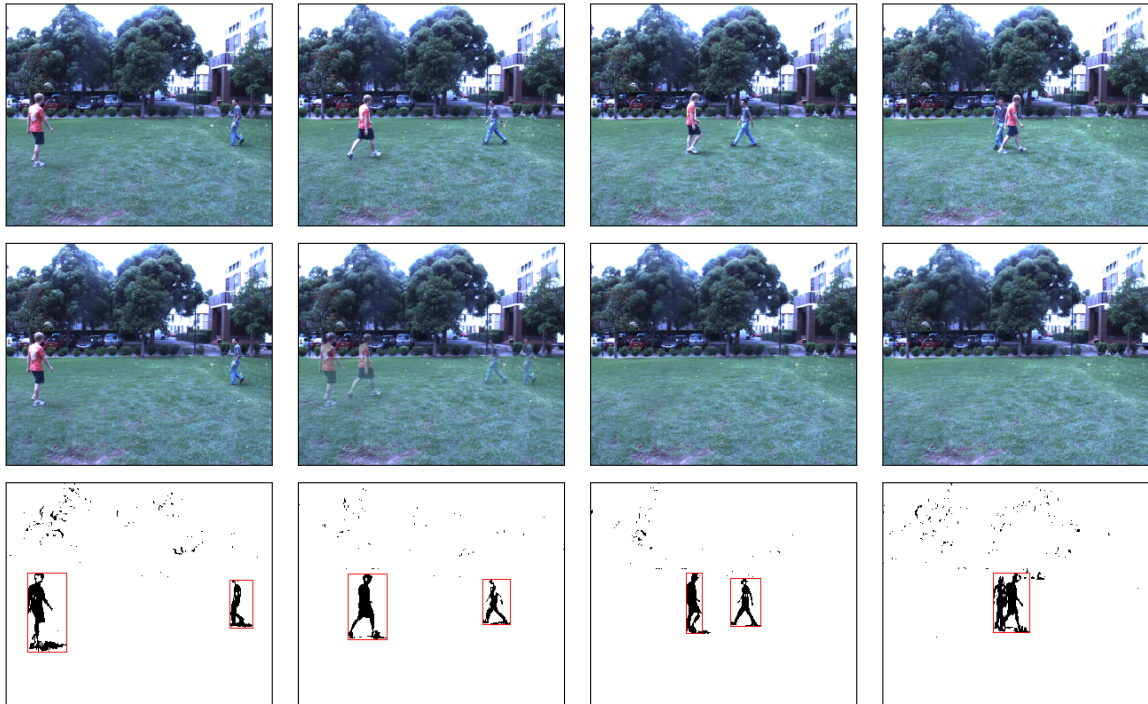
Figure 2.4 – Object detection using a background model. Top row: input image sequence. Middle row: background images obtained via median filtering (image in n^{\text{th}} column is result of filtering input images 1 to n ). After only four images, the foreground objects have been completely removed. Bottom row: Objects detected by comparing each input image to the final background image.
