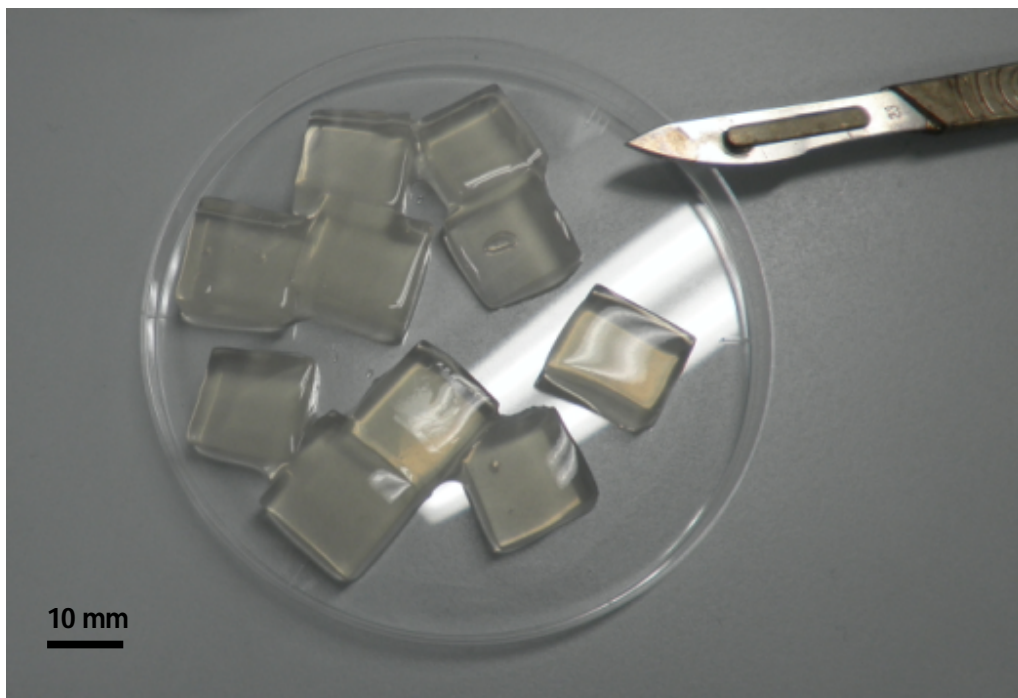
Figure 33. Agar cubes cut with scalpel to scaffold dimensions
