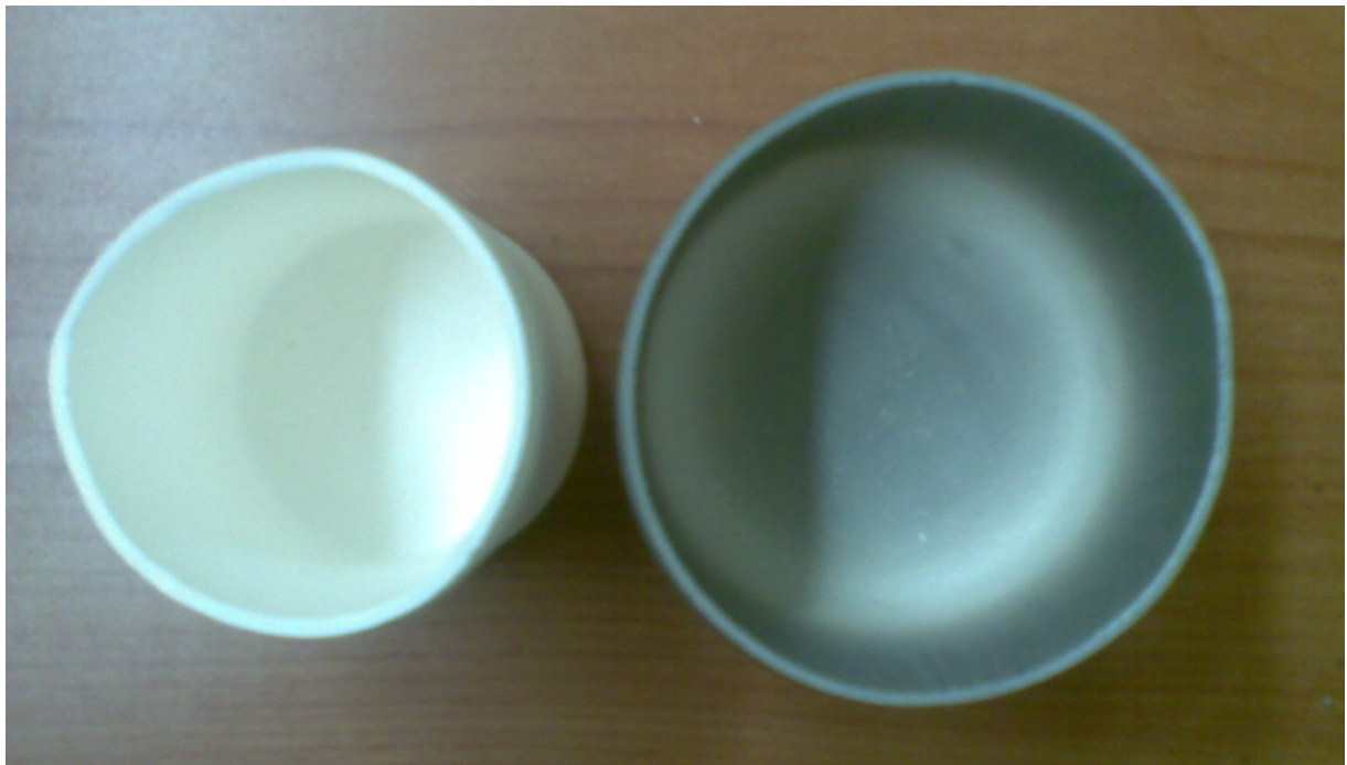
Figure 54. Platinum sputter-coated alumina crucible. Left: An un-coated alumina crucible. Right: A platinum coated crucible – incomplete coating can be seen on the edges on the base.
