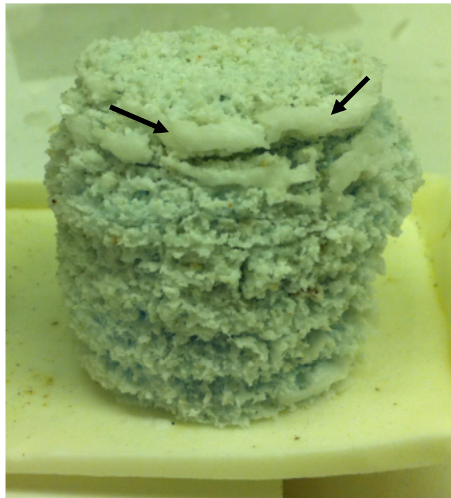
Figure 51. Pellet calcined at 1150°C. Glassy formation is indicated by arrows.
