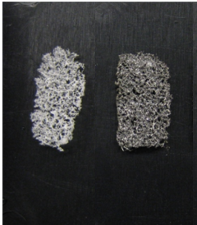
Figure 59. Left: Un-coated scaffold slice. Right: BMG sputter coated scaffold slice.
