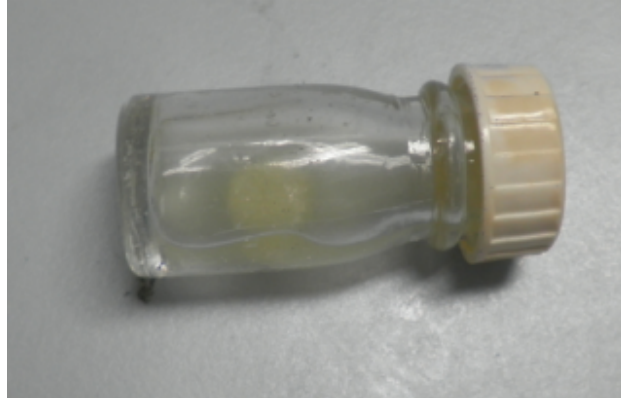
Figure 67. Scaffold turned yellow after 24 hours in the presence of NBB4. This is due to NBB4 adhering to the scaffold.
