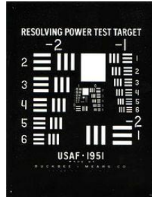
Fig.14. An example of resolution test chart (1954 USAF). This 1954 USAF was set by US Air Force.
