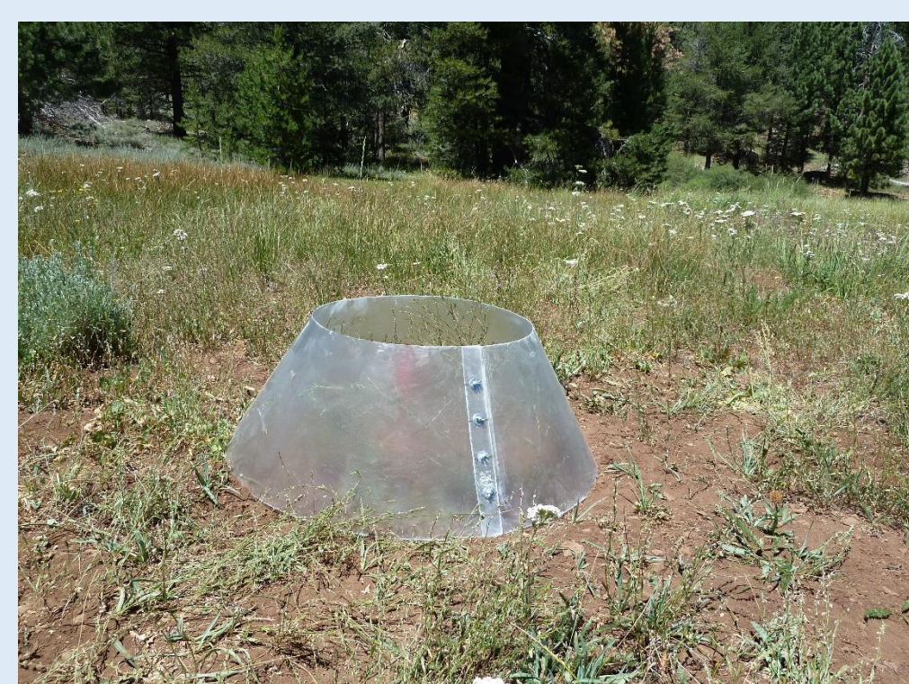
Figure 2. Open top perspex cone used to passively heat ground-dwelling wasp nests. Based on Holway (1996). Photo: L. Yang
