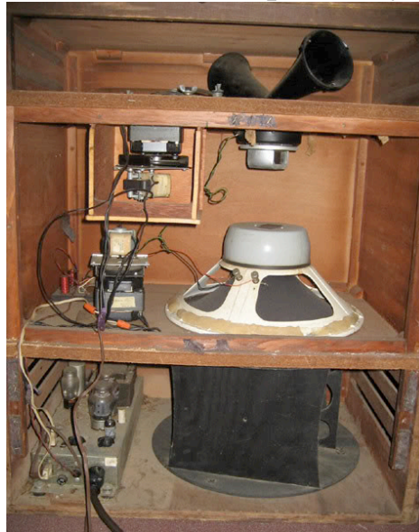
[Figure 2]: The components inside a Leslie speaker cabinet. Sourced from Tumblr
