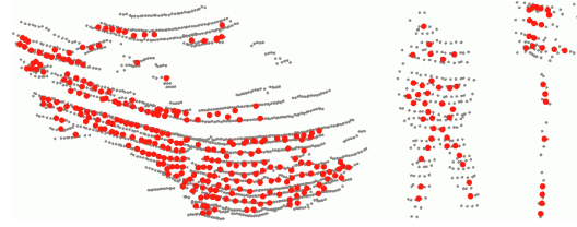
Figure 3.13 – Keypoints at flat or linear regions on a car, pedestrian and sign.
