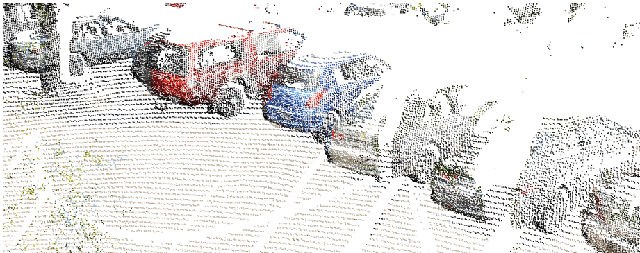
Figure 2.5 – A dense, coloured RIEGL scan of a car park.
