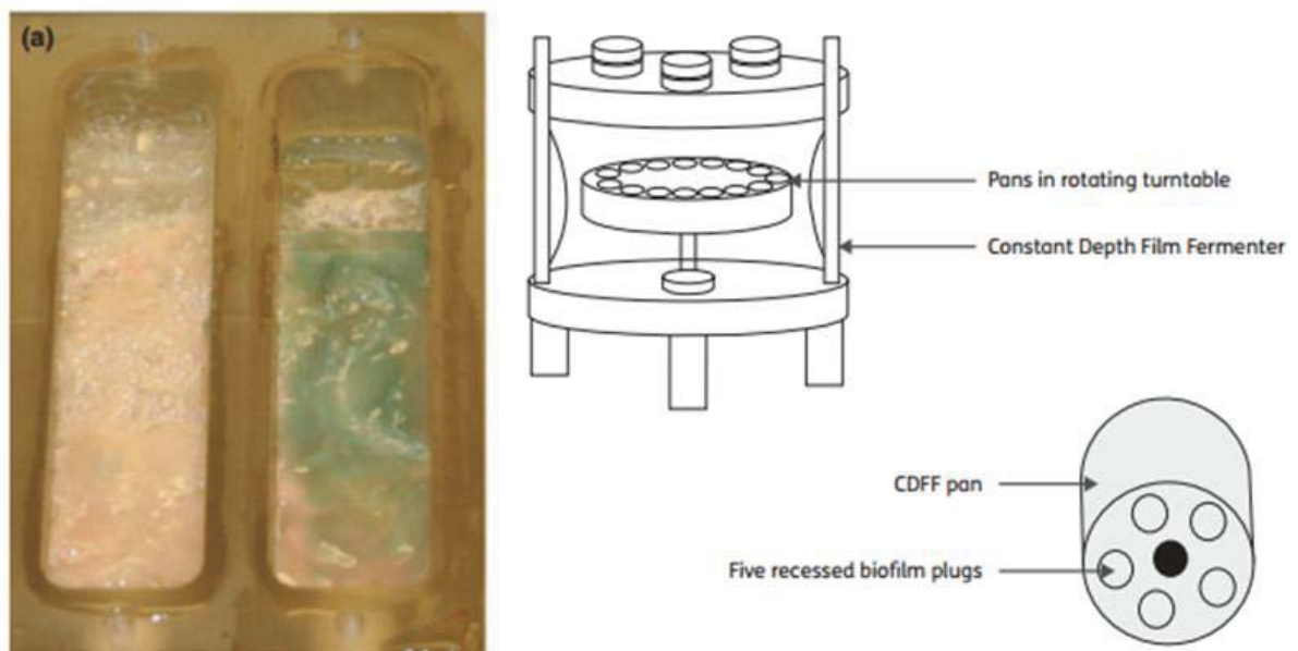
Figure 1.8: Left: Drip-flow reactor model (Woods et al.) Right: CDFF with plug inserts (Hill et al) [158].
