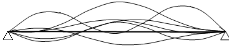
Figure 5-2: Example of random shape of initial out-of-straightness for a simply-supported column
