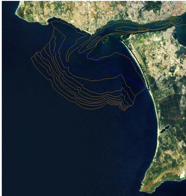
Figure 4.12 - Modelled bay shape planform for the northern sub cell after adopted wave rotation.
