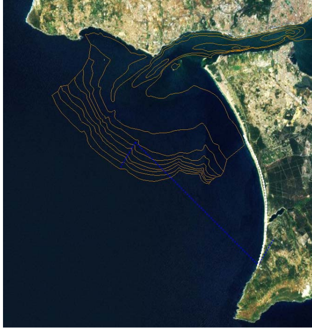
Figure 4.11 - Modelled bay shape planform for the southern sub cell after adopted wave rotation.
