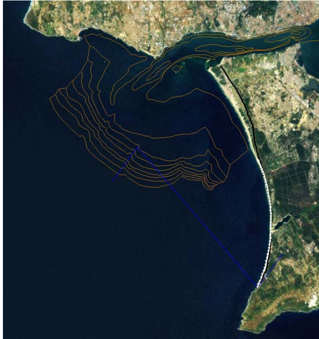
Figure 4.21 - Wave climate rotation ( 7^{\circ} counter clockwise) required for a best fit of the bay shape planform with the paleo coastline inferred for climbing dune formation in the southern sub cell (black line represents coastline position at the time).
