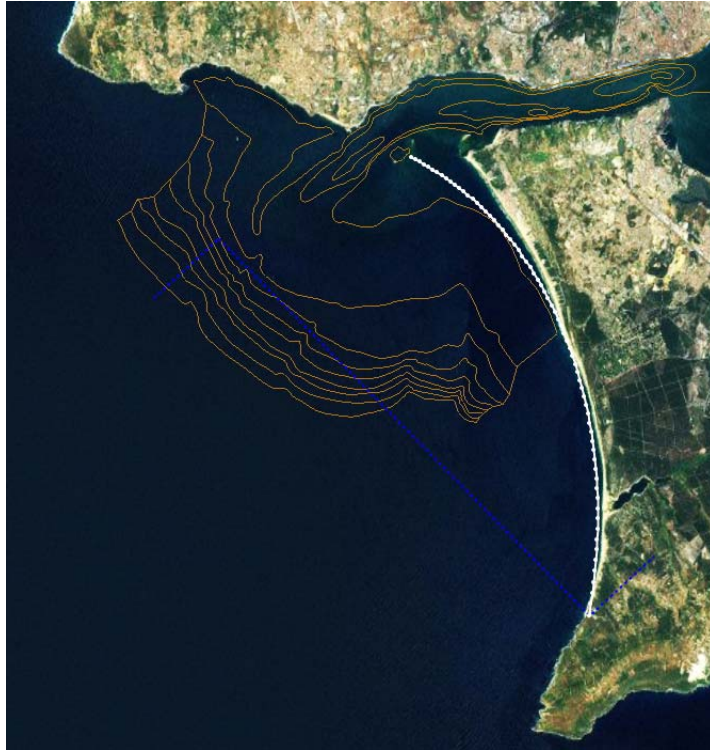
Figure 4.5 - Modelled bay shape planform compared with the present coastline of the entire Caparica coastal cell.
