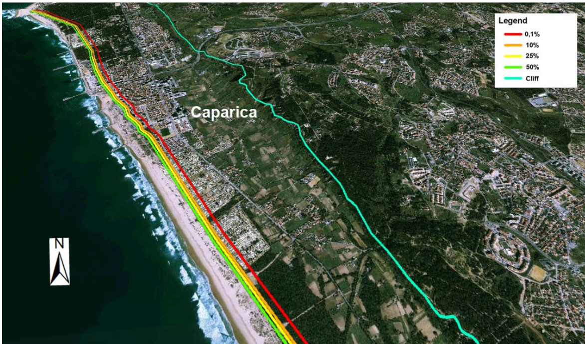
Figure 5.24 - Risk contours for the 2050 forecast indicating the extent of recession for different probabilities of exceedence.
