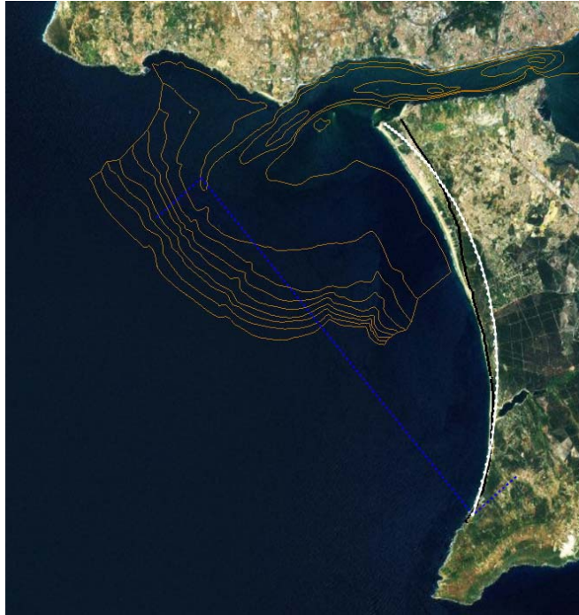
Figure 4.18 - Updrift control point relocation due to modified delta bathymetry required for a best fit of the bay shape planform with the coastline location inferred for the period when climbing dunes were active (black line represents coastline position at the time).
