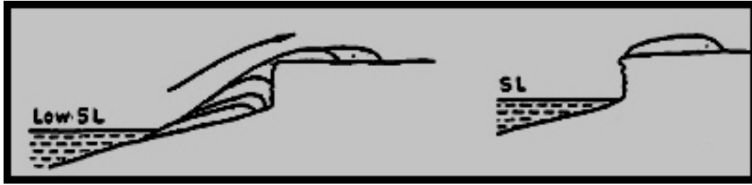
Figure 3.2 - Schematic diagram of cliff-top dunes development (Adapted from Jennings, 1967).
