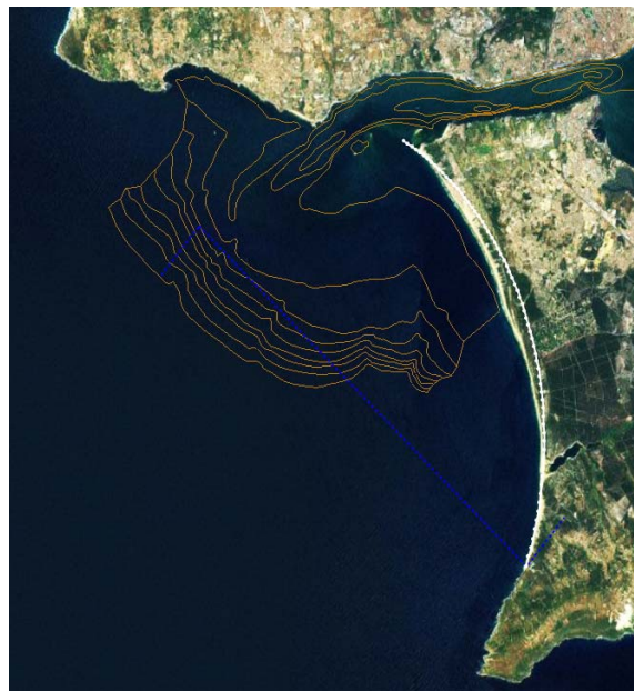
Figure 4.10 - Modelled bay shape planform compared with the present coastline after adopted wave rotation.
