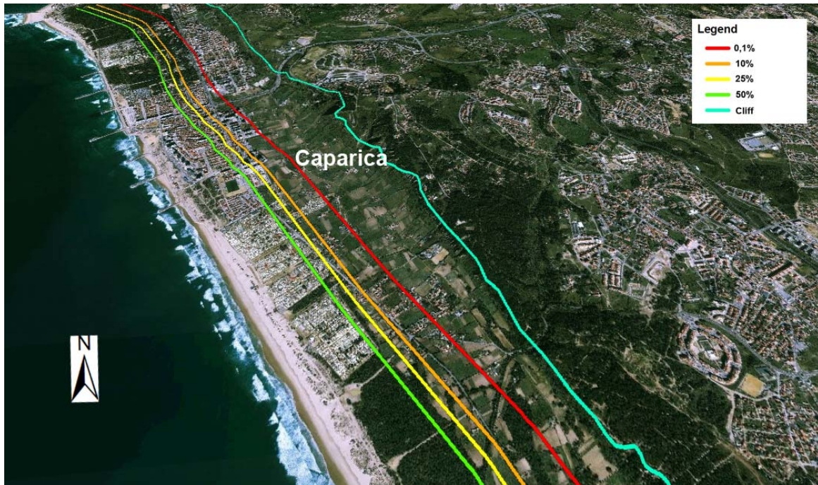
Figure 5.25 - Risk contours for the 2100 forecast indicating the extent of recession for different probabilities of exceedence.
