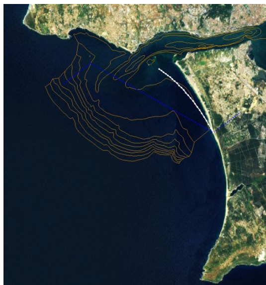
Figure 4.16 - Modelled bay shape planform for the northern sub cell after adopted wave rotation.
