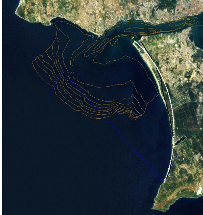
Figure 4.17 - Wave-climate rotation ( 25^{\circ} counter clockwise) required for a best fit of the bay-shape planform position to the coastline location inferred for the period when climbing dunes were active (black line represents coastline position at the time).
