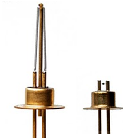
Plate 3-1 Example of a TCD filament (left) and a thermistor bead on the right. (Source: AGC Instruments)
