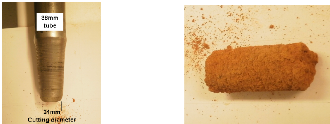
Plates 4-1 Close-up of the corer cutting edge (a) used to recover soil plugs (b) with dimensions 24mm across and lengths to 500mm which were very suitable for the SCB.
