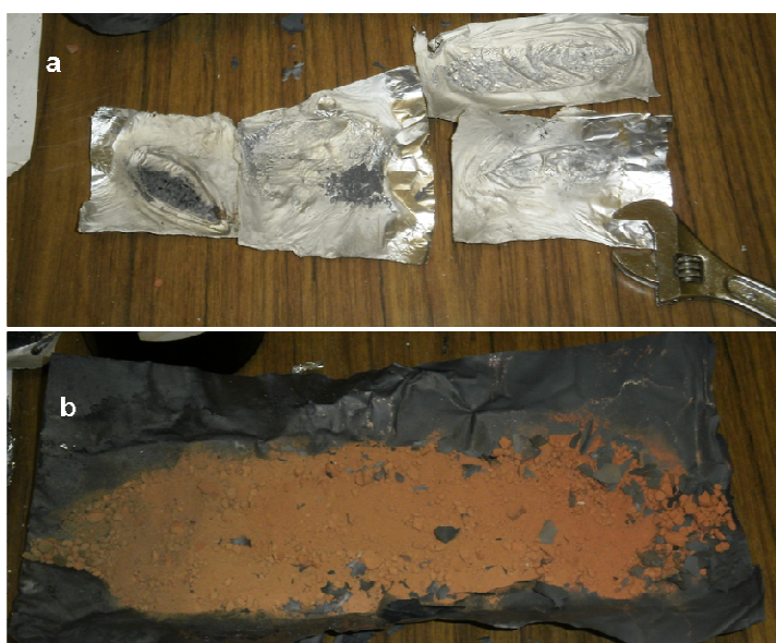
Plate 3-3 Combustion of charcoal on foil (a) and soil (b) under variable O 2 conditions.
