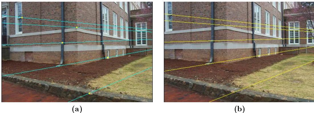
Figure 2.20 – Example of epipolar lines. For each point in (a) there is an epipolar line defined in (b), and it is possible to see that each of these lines pass on their corresponding points in the other image (these points were selected manually, without a corresponding match).
