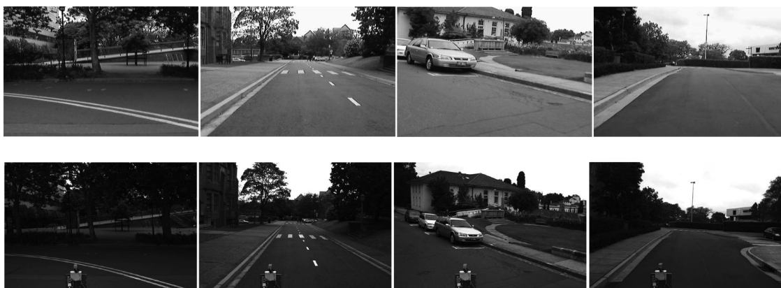
Figure 4.12 – Examples of images taken at the same vehicle position with different cameras. The first row corresponds to the original camera and the second row corresponds to the new camera (the new camera can be seen in the images captured by the original camera). The displacement between cameras is approximately 1.4 m horizontally and 0.5 m vertically, with a pitch change of roughly 10^\circ .
