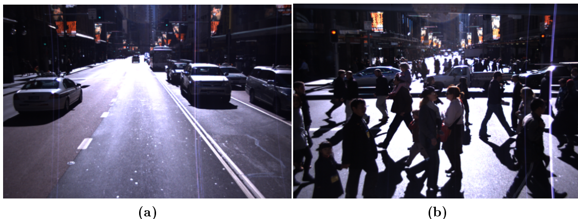
Figure 5.1 – Examples of dynamic objects in visual odometry. (a) Constant flux of cars in one portion of the image, generating a contrary optical flow that creates systematic drift. (b) Pedestrians crossing the vehicle's path while it is not moving, generating random optical flow that compromises orientation.
