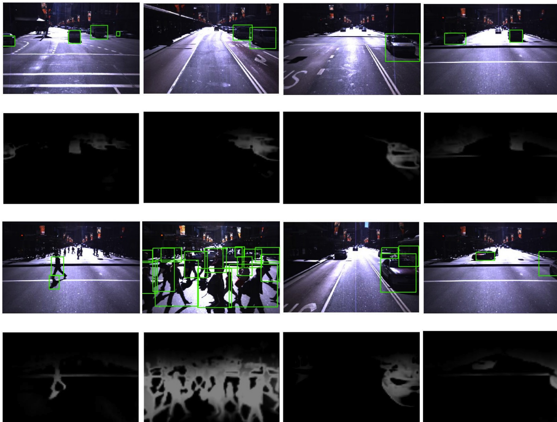
Figure 5.13 – Different objects obtained during the segmentation process.
