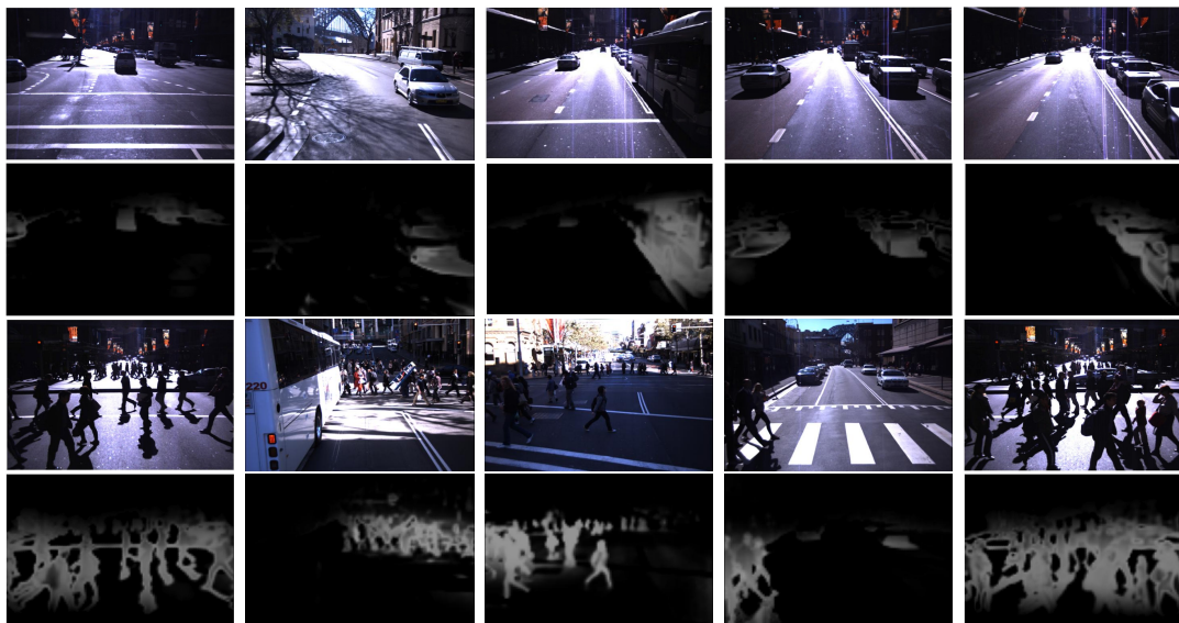
Figure 5.10 – Automatic dynamic object segmentation results. Each pixel is defined by a number ranging from 0 (black, static object) to 1 (white, dynamic object). These results were obtained in the same run as the non-parametric model constantly adapts to new environment characteristics, without any prior information and without any human intervention.
