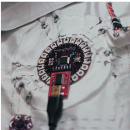
Fig. 4. The Lilypad Arduino is one of the microcontrollers used in Wo.Defy. (Photo © Emily Ip.)
